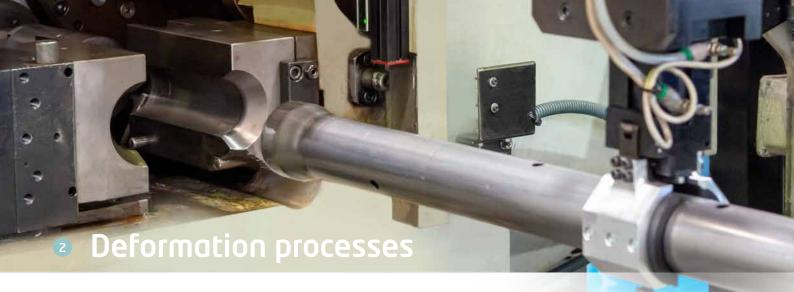
We apply deformations in the tubes, either by reductions / expansions at the tube ends, or using dies and presses to directly supply to the assembly plant, without the need for additional processing.
