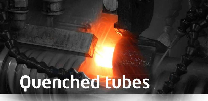
Induction quenching is based on the material heating while passing through a high strength variable magnetic flield. Heating penetration depends on working frequency. An accurate control on it ensures a perfect quenching homo-
